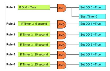
Figure 8.26 GCL Logic for Sequence Control (Turns On in Sequence and Remains On)
