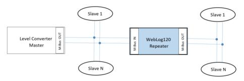
The M-Bus line of the existing master or level converter is connected to the terminals marked M-Bus Repeater. As standardized for M-Bus slaves, the polarity is arbitrary. A processed signal for connecting an M-Bus network is then available at the M-Bus output of the WebLog120. This M-Bus network can then be read out by the WebLog120 and the other master one after the other, but not at the same time.
