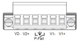
Wire Gauge: 12 - 24 AWG (3.31 - 0.205 mm) Torque: 7 1b-in
